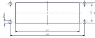
Panel cut-out for wall thickness 1.5 - 2 mm (for snap-on attachment)
